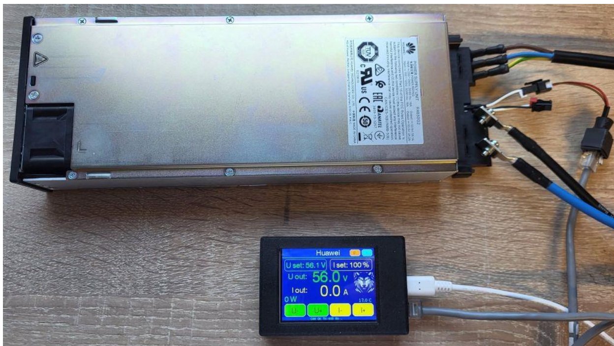
CAN-GO X with a Huawei rectifier, USB-C power and CAN communication.
